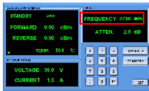
[Picture 5.] Frequency setting complete
